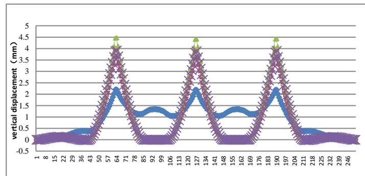
**Figure 11** Track Slab Displacement under Three Narrow Joints' Failure
