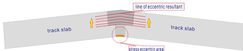
Figure 6 Eccentric Resultant in the Joint
