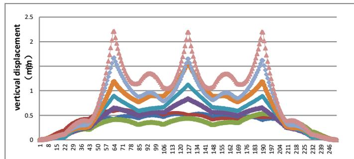
**Figure 10** Track Slab Displacement under Joint's Three Uneven Damage
