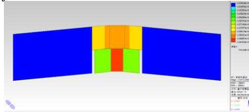
Figure 5. Stress Concentration at Bottom of Joint Concrete
