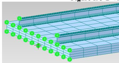
Figure 2 Fixed Constraints at Segment Ends
