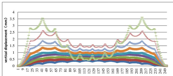
Figure 8. Track Slab Displacement under Joint's Different Even Damage
