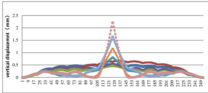
**Figure 9** Track Slab Displacement under Joint's Single Uneven Damage
