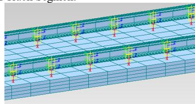
Figure 3 Rail fasteners constraints
